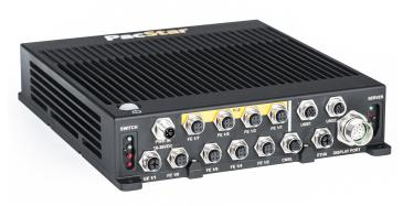
PacStar 551 provides high-performance compute and switching services for critical voice/ video, data, application or virtual network function hosting in a compact, rugged form factor. The PacStar 551 is based on Intel® computing and Cisco<sup>®</sup> switching technology and provides up nine switched ports.
